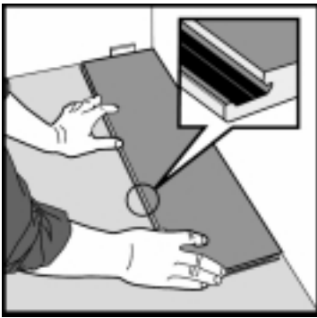
Fig 1. First plank, first row. Start in a left-hand corner of the room with the locking strip (groove) facing the room. Remember to leave a gap between the wall (left) and the board. It is practical to adjust the gap between the long sides and the wall later, when three rows have been installed.
