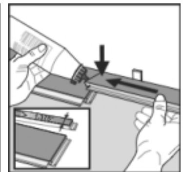
Fig 12. Joining length cut panels. First/last row(s). Glue the joint with white glue, put a weight over until the glue has hardened.
