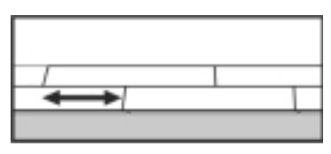
Fig 8. General. Minimum distance between short ends of planks in parallel rows shall not be less than 9" or half the distance of the plank.
