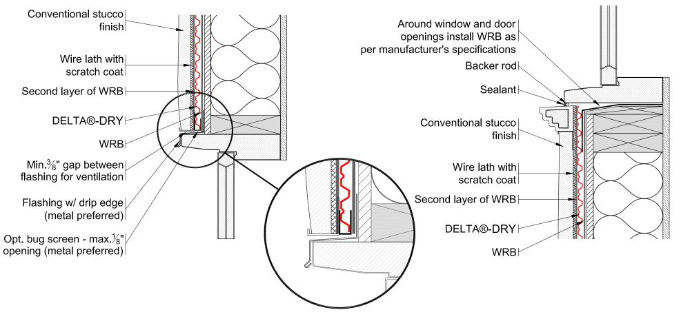
$^{\circ}$  For proper performance of DELTA®-DRY ensure top and bottom remain open to allow ventilation and drainage  $^{**}$
