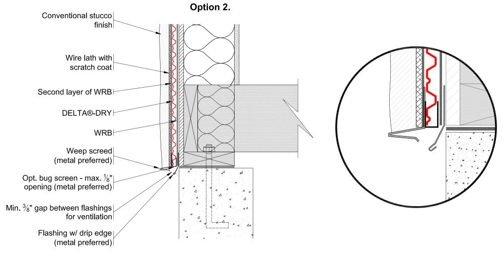
$^st$  For proper performance of DELTA®-DRY ensure top and bottom remain open to allow ventilation and drainage  $^{stst}$
