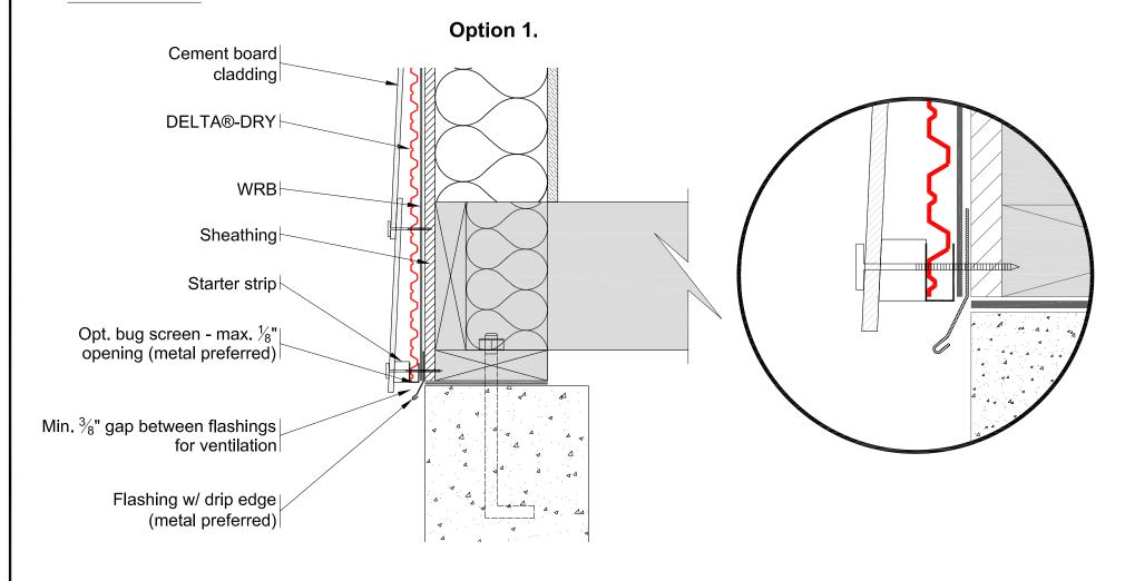
$^st$  For proper performance of DELTA®-DRY ensure top and bottom remain open to allow ventilation and drainage  $^{stst}$
