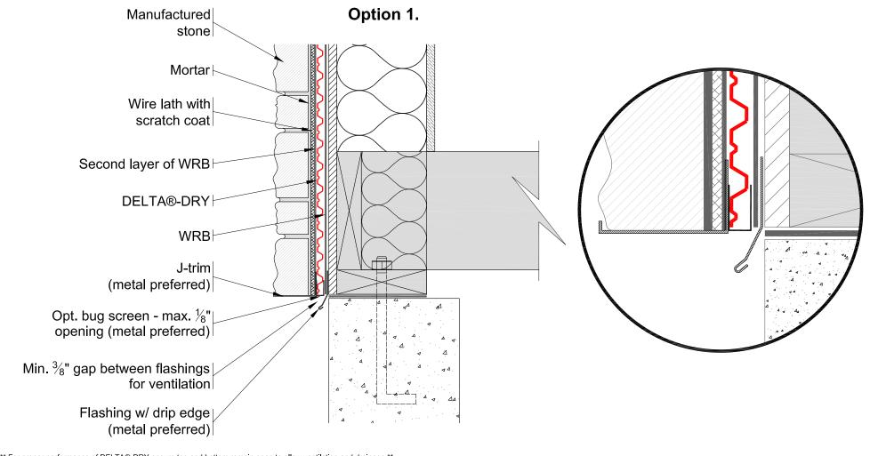
\*\* For proper performance of DELTA®-DRY ensure top and bottom remain open to allow ventilation and drainage \*\*
